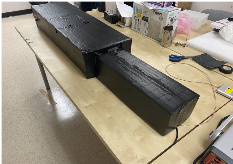
Figure 7: The FORMOSA PMT testing dark box. A doubly layered cardboard arrangement with thick tape covering all external surfaces of each layer. Can comfortably accommodate a 1m x 5cm scintillator bar with PMT pressed up against it.
