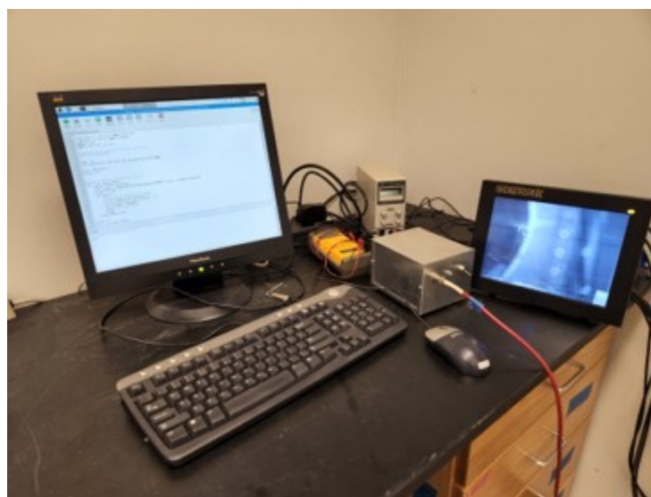
Figure 6: An image of the setup to externally control and view the motion stage while under vacuum.
