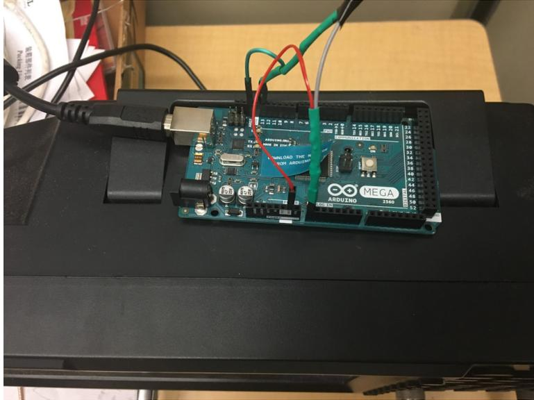
Figure 10: The Arduino based temperature collection system. The actual probe was placed on top of the shielded room close to an exhaust fan.
