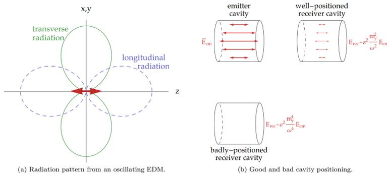
Figure 2: (a) shows the radiation pattern for transverse and longitudinal modes of an electric dipole. (b) shows the positioning of a detector that would permit the maximum field to penetrate. Image from [5]
