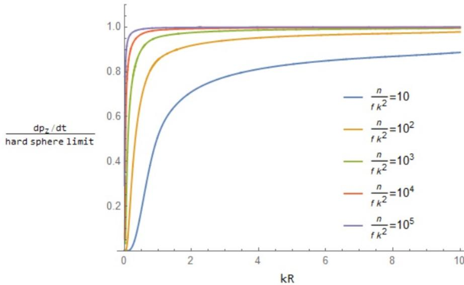
Figure 3: Ratio of force with a finite potential and force in hard sphere approximation. The force approaches the hard sphere limit as the radius of the scattering object increases.
