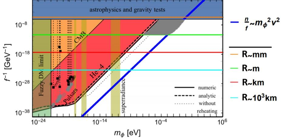
Figure 4: Exclusion plot for light dark matter particle candidate. The region to the left of the diagonal line has a scattering potential. The horizontal lines indicate the radius required to be able to use the hard sphere approximation. The proposed experiment should be sensitive to the region shaded in grey.
