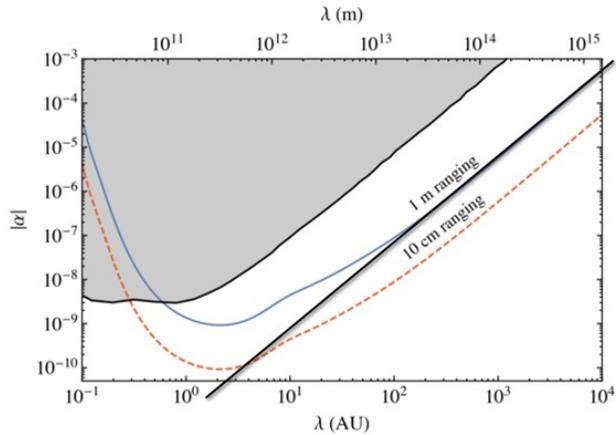
Figure 5: Sensitivity plot for the proposed experiment. The shaded region indicates the excluded values for the Yukawa potential. The blue solid line indicates the conservative sensitivity of the experiment, while the red dashed line indicates the optimistic sensitivity. The straight black line is added to emphasize the linear region of the sensitivity.
