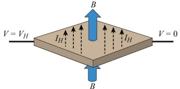
Figure 10. Hall Effect Measurement Example
