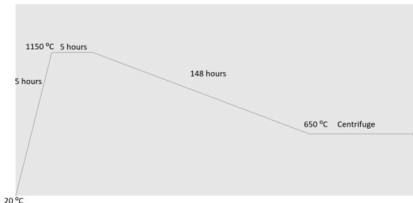
Figure 3. Temperature profile for  $\text{CeCoGe}_3$  reaction.
