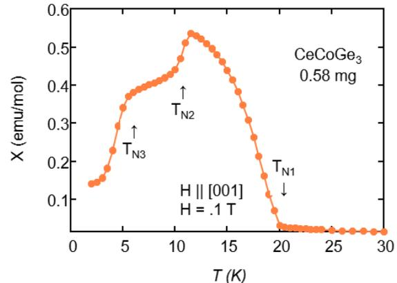
Figure 7. Magnetic Susceptibility vs. Temperature showing three Neel transitions.
