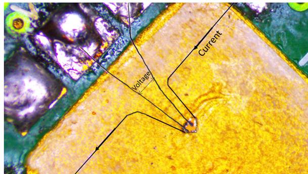
Figure 4. Resistivity measurement along the  $[100]$  axis.
