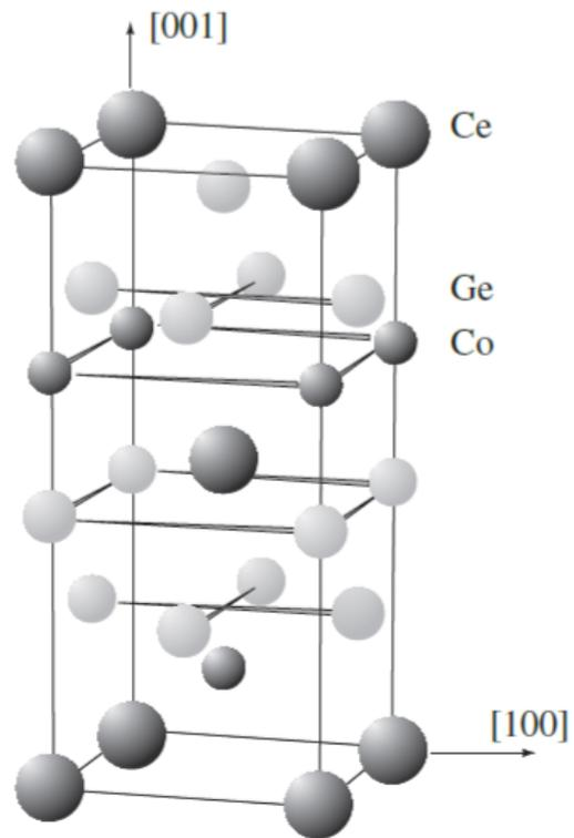
Figure 1. Crystal Structure of CeCoGe<sub>3</sub>.
