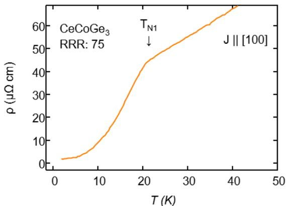
Figure 6. Resistivity vs. Temperature showing Néel transition at 21 K.
