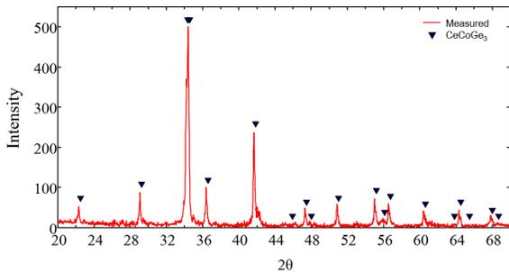
Figure 5. Powder X-Ray Diffraction of  $\text{CeCoGe}_3$ .
