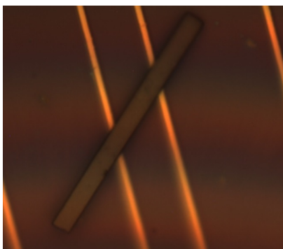
FIG. 2: 100X magnification of a typical \text{MAPbI}_3 device. The small gap between the electrodes is close to 8\ \mu\text{m} in length and the large gaps are close to 20\ \mu\text{m} in length.
