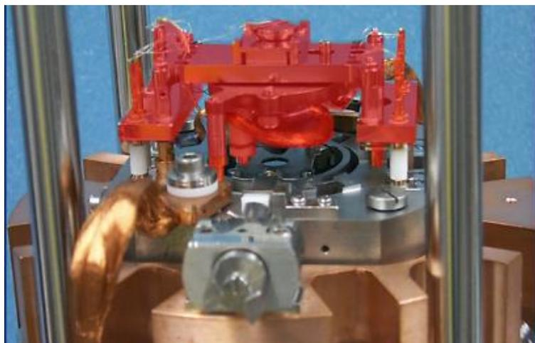
**Figure 6.** The mechanical setup of the STM inside the vacuum chamber. The scanner, shown in red, can be removed from the chamber to allow tip replacements. A sample holder can be seen below the scanner, although the scanner's tip is too small to be visible. [1]
