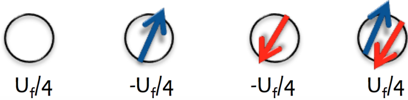
Figure 7: The potential induced on a localized site to induce local moments. The blue arrow denotes a spin up electron, while the red arrow denotes a spin down electron.
