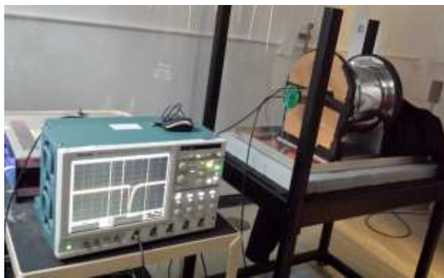
Figure 13: Image of testing NaI scintillator with PMT and oscilloscope.
