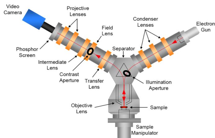
Figure 2: Elmitec LEEM III. Electron path is shown in red. Both the electron source and the sample are at a potential of -20kV, while all the lenses are at ground potential. The sample has an additional voltage which determines the energy of the incoming electrons. [6]
