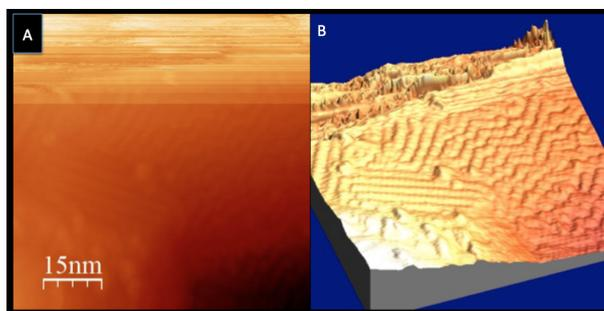
Figure 4: STM images of cleaned Ge(110) at room temperature. (A) Raw image. (B) 3D model created by STM analysis software. In (B) the zigzag configurations of the atoms show a  $c(8 \times 10)$  reconstruction, and the rows on the left appear to have the  $(16 \times 2)$  reconstruction. (Diagram in Figure 1)
