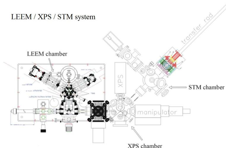
Figure 3: Configuration of LEEM/XPS/STM system. All chambers are under ultrahigh vacuum. Sample transportation was accomplished using two magnetic transfer rods. Samples are put into the system using a small entry chamber attached to the STM. [7]
