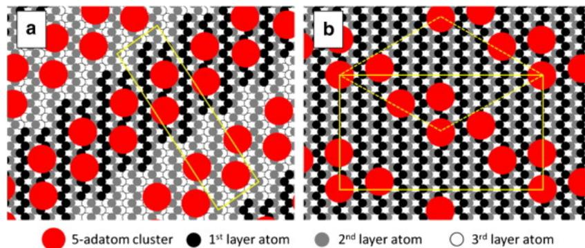
Figure 1: Diagram of both the common reconstructions of Ge (110) with the unit cell outlined in yellow. (a) In the  $(16 \times 2)$  reconstruction, the underlying surface atoms alternate between missing a layer of Ge(110). (b) In the  $c(8 \times 10)$  reconstruction, all of the 5-adatom clusters sit on the same plane.[3]
