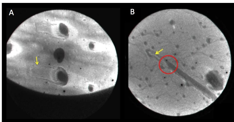
Figure 8: Island traces observed with LEEM once the Ge(110) sample had cooled down. Yellow arrows point to the traces left on the Ge(110) surface. The red circle marks the end of the Ag island. (A) Shows the trace left behind by Au. Outlines can be seen around the remaining circular islands that resemble the 1D islands formed at high temperatures. (B) Previously observed "trails" left behind by Ag after contraction.[5]
