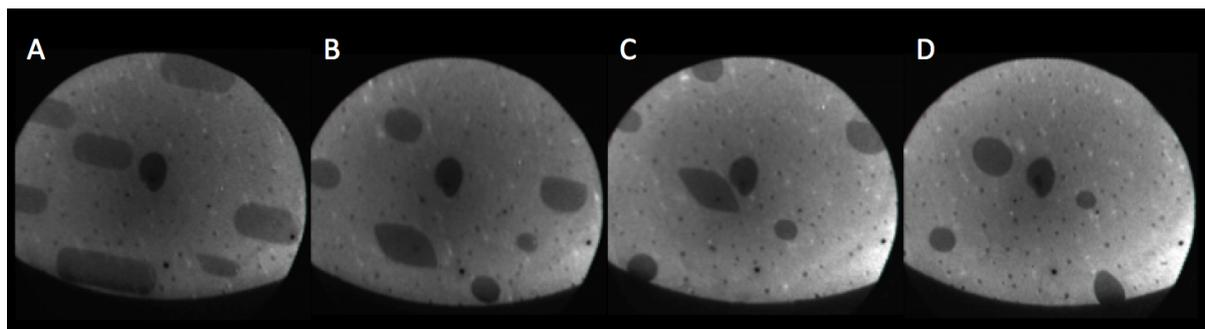
Figure 7: Island contraction seen with LEEM. As the surface temperature decreases, islands rapidly contract into more circular structures. Image (A) shows islands at maximum temperature (825 °C). As the sample cools, the islands reform into those seen in (B). Images (C) and (D) highlight the rapid reforming of the oval island in image (C) into the circular island seen in (D).
