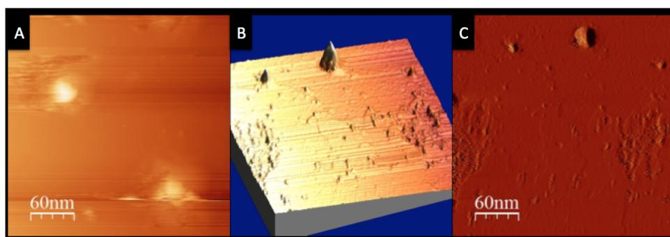
Figure 5: STM images of mound-like structures found on a cleaned Ge(110) surface at room temperature. Image (B) is the 3D model of (C) generated by the analysis software. Image (C) is a derivative image generated from the raw image. In (C), darker areas correspond to a steeper gradient. (B) contain two smaller mounds which could get larger with more sputtering.
