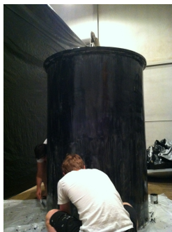
FIG. 13. Painting the detector with black
