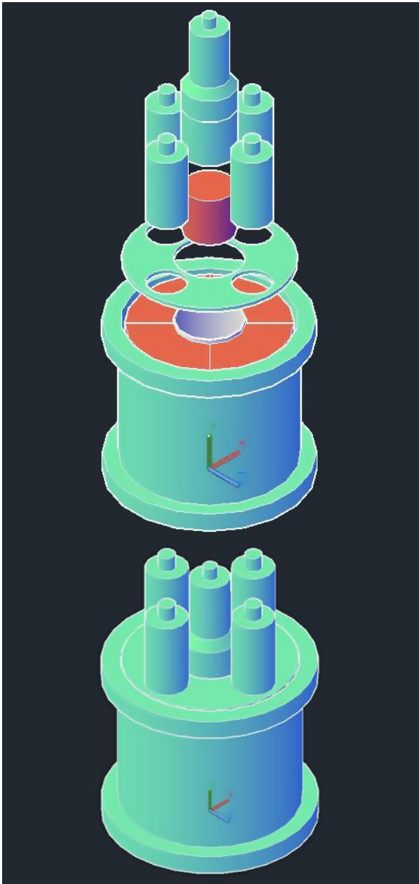
FIG. 6. Render of CAD drawing of NaI detector assembly. Top is disassembled assembly to display hidden components.
