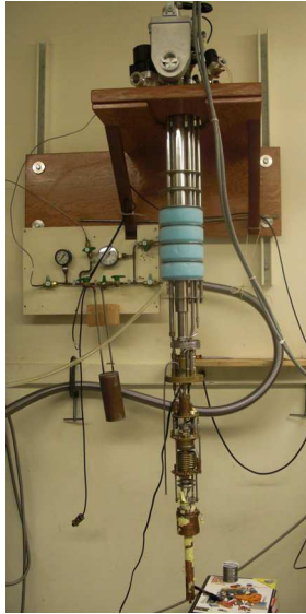
FIG. 4: The dilution refrigerator used in taking data
