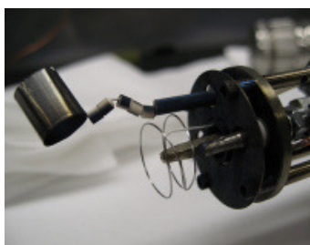
Figure 5: The electron beam-evaporator mechanism which doses the sample with metal. In the center is a rod composed of the metal to be dosed or a tungsten rod with a layer of that metal wrapped around it. The circular tungsten filament provides electrons when heated. Those electrons are accelerated by an attractive voltage onto the metal to be dosed, causing it to vaporize and hit the germanium sample. When placed in front of the rod, the cylindrical foil is used to measure the amount of metal that is being evaporated
