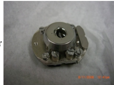
Figure 4: The sample holder that allows us to move the germanium sample from chamber to chamber within the UHV system. The sample sits under the circular opening of the top plate of the holder.
